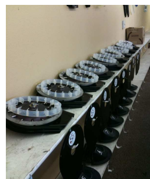
Precision Planting meters with SureFire seed belts cleaned and waiting to be re-assembled.
